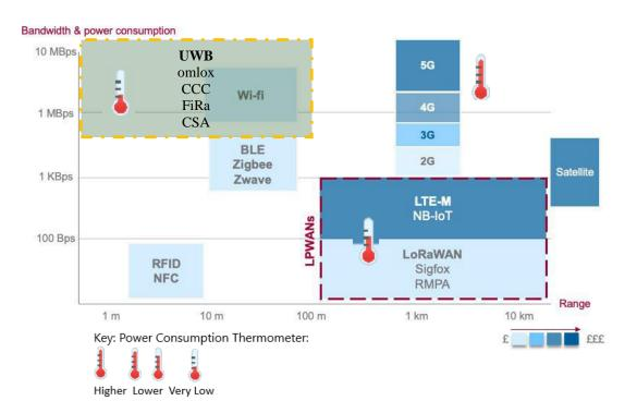
UWB does not completely fit the traditional trade-off between bandwidth, data rate and power consumption. We've added the thermometer icon to the figure above to depict power consumption. UWB can deliver moderate data rates at very low power consumption – closer to RFID and NFC and typically much lower than NB-IoT or LoRaWAN.
